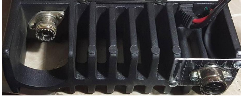
Carrier Detect signal port at the Yaesu FT-2900
